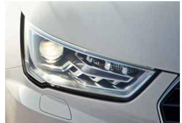
Xenon headlights with LED daytime running lights
