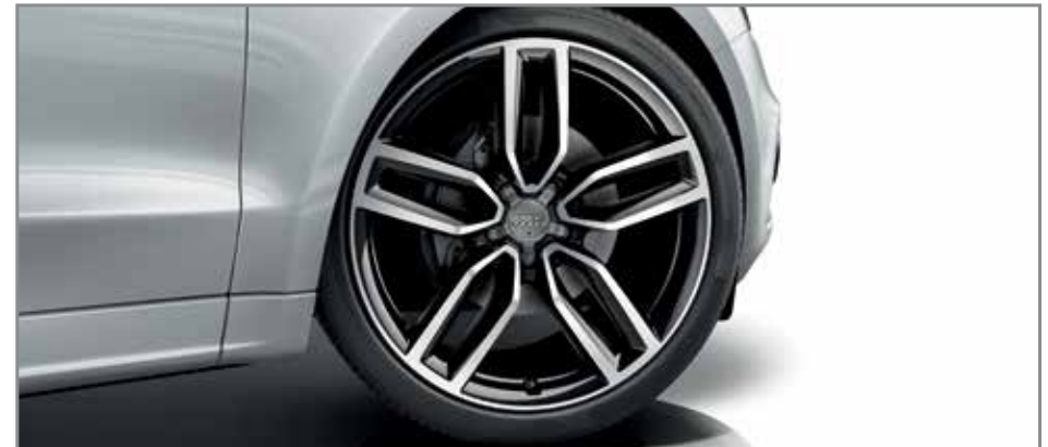
21" x 8.5J '5-twin-spoke-star' design alloy wheels in black with 255/40 R21 tyres (PQ1)
