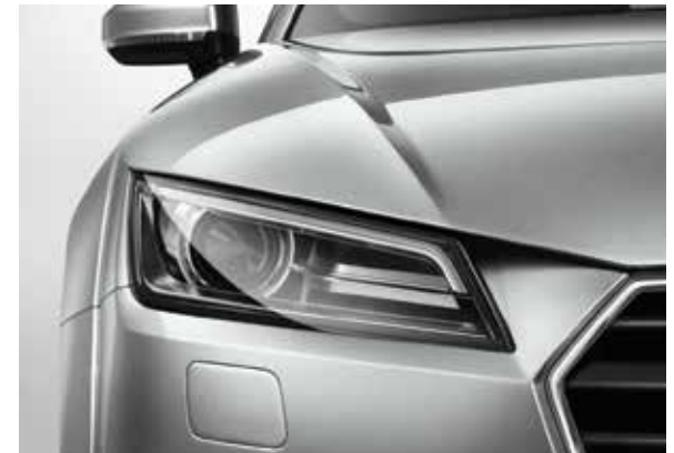
Xenon headlight with LED daytime-running light
