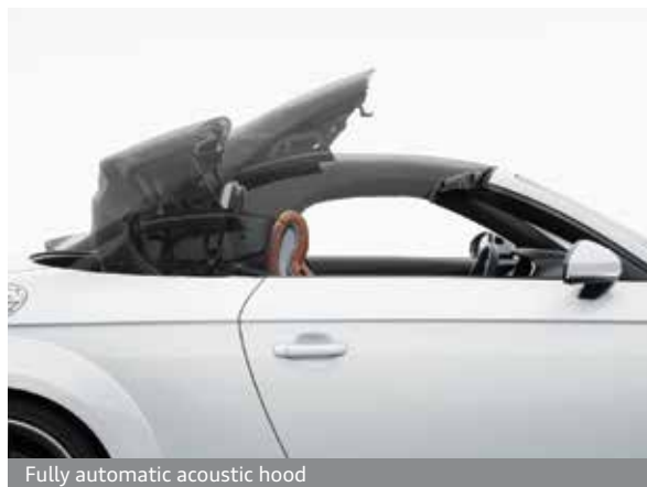
Fully automatic acoustic hood
