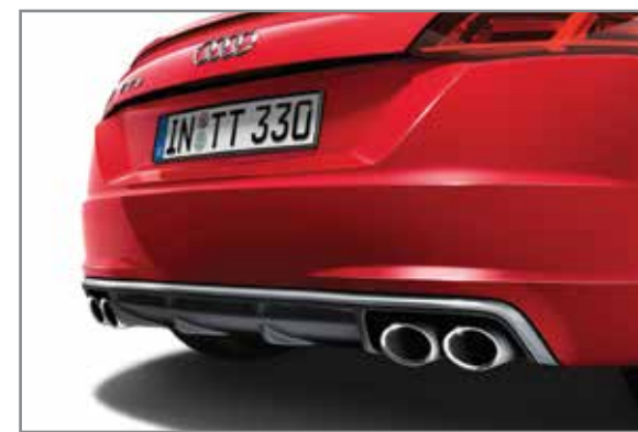
TTS rear bumper incorporates a diffuser insert in Platinum grey with a surround in aluminium look
